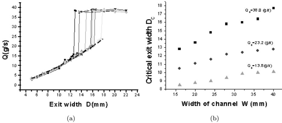
Fig. 2. (a) At a fixed inflow rate  $Q_0$ , the relation between the outflow rate  $Q$  and the exit width  $D$  in different width of channel. From left to right, the width of channel  $W$  are corresponding to 16, 20, 24, 28, 32, 36 and 40 mm. (b) there is a different critical exit width  $D_c$  for the different inflow rate  $Q_0$  in the same width of channel  $W$
