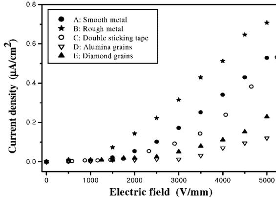
Fig. 2. The variation of current density vs. electric field measured with different electrodes.
