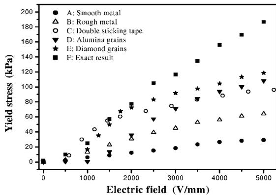
Fig. 1. The variation of yield stress vs. electric field measured with different electrodes.
