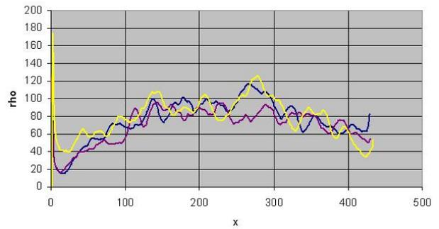
**Fig. 4b** density profile in 2d cell. Blue & pink: cell moving towards negative x (the left); yellow: cell moving towards positive x ( the right); x is the direction of vibration; it is in pixels with 450pixels $\approx$ 29mm; rho or r(x) stand for density in a.u..
