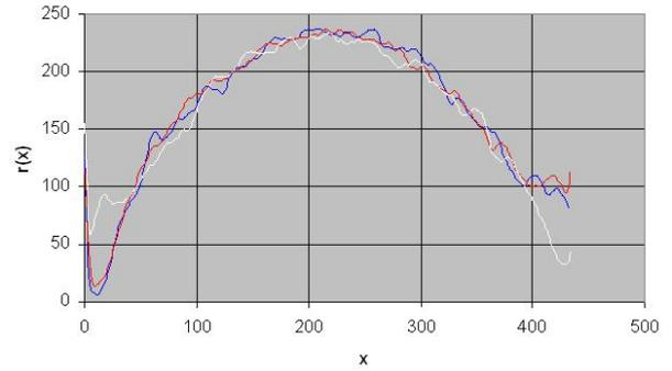
**Fig. 4a** density of cluster profile in the direction of vibration. Red and blue: cell moving towards negative x (the left); white: cell moving towards positive x (the right).
