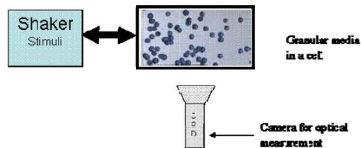
**Fig. 1** typical experimental set-up. The camera shall allow 3-d diagnostic at 1000 frames/s
