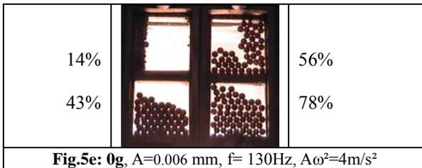
**Fig. 5** Chinese satellite cell in Airbus; gravity direction is horizontal (when it is different from 0); vibration direction is horizontal. Area fractions for the 4 cells are 43%, 56%, 78% and for the large particle in the mixture is 14%, as indicated in Fig5.e.
