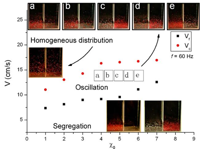
FIG. 1 (color online). The phase diagram for the homogenous (HS), oscillatory (OS), and segregated (SS) states. See the captions of Figs. 3 and 4 for the uncertainties in  $v_c$  and  $v_f$ . Also shown are the photographs of the configurations of the system with glass beads being darker (red) and steel balls being lighter (silver). Snapshots (a)–(e) are taken during one cycle of the clock. Note that  $f = 60$  Hz and the period of the clock (Fig. 4) can range from tens to hundreds of seconds.
