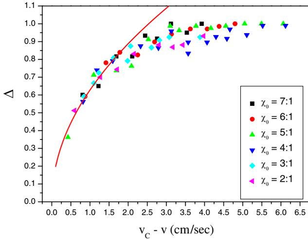
FIG. 3 (color online). Variation of oscillation amplitude  $\Delta$  as a function of distance away from the critical velocity ( $v_c - v$ ) for various  $\chi_0$ . The solid line is a fit of the data to the form  $\Delta \sim (v_c - v)^{1/2}$  for small  $v_c - v$  with  $v_c$  being adjusted within 20% of the experimental observation to give the best fit. Uncertainties of the data are smaller than the size of the symbols.
