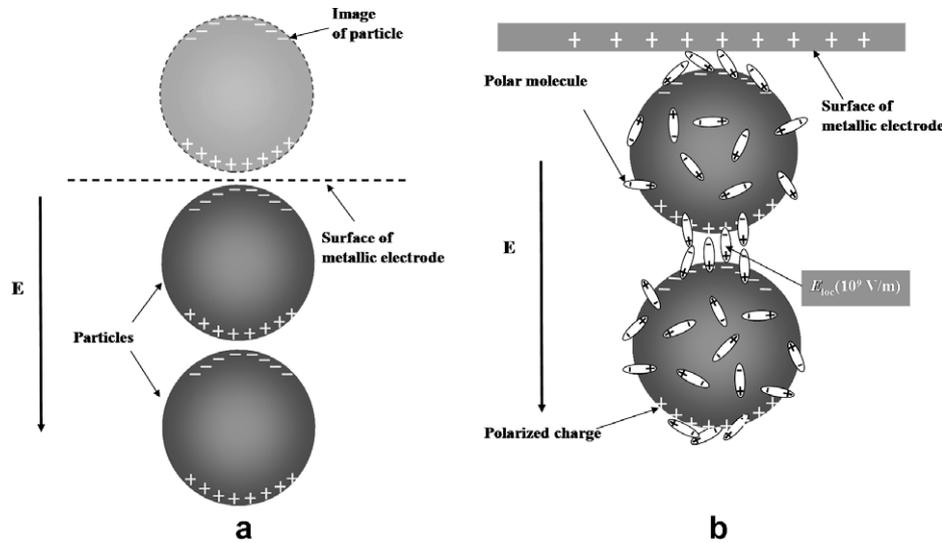
Fig. 1. Scheme of particles and metallic electrodes (a) in conventional ER fluids and (b) in PM-ER fluids.
