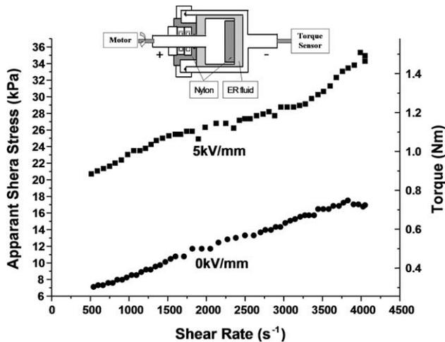
Fig. 3. Dependence of the apparent shear stress on the shear rate under different electric field. Upper inset is a configuration of the sealed cylindrical rheometer.
