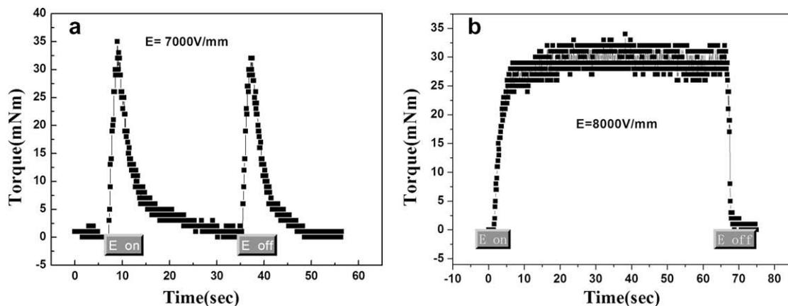
Fig. 4. The feature of the torque measurements using the electrodes covered by an insulating tape for ER fluid with ions contained (a) and without ions contained (b).
