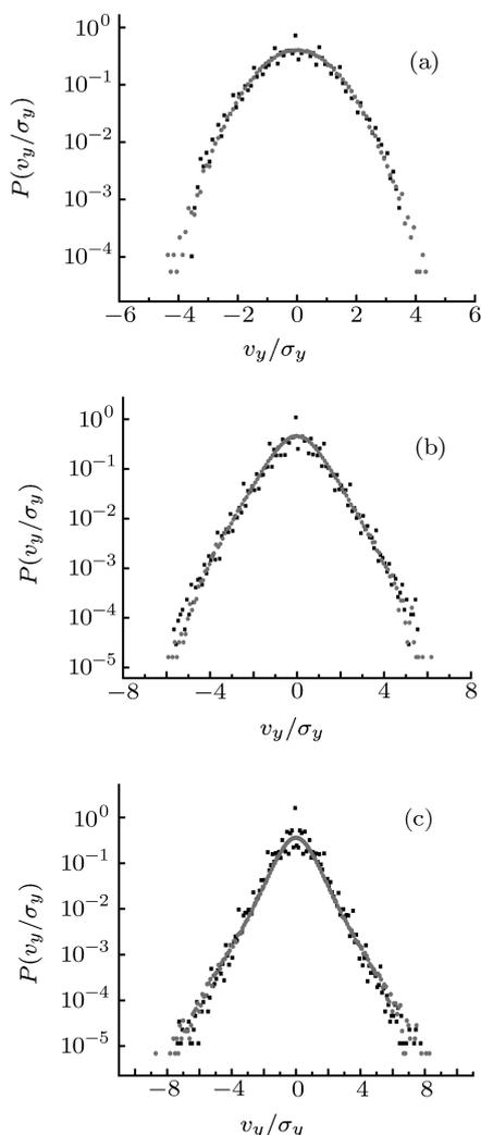
**Fig. 5.** Velocity distribution curves with fitting function  $P(v_y) = C \exp[-\beta(|v_y|/\sigma_y)^\alpha]$ , obtained from the simulation of 2, 6 and 10 layers respectively where black rectangles denote experimental results, gray circles represent simulation results, (a)  $\alpha = 2.0$  for two layers, (b)  $\alpha = 1.45$  for six layers, and (c)  $\alpha = 1.25$  for ten layers.
