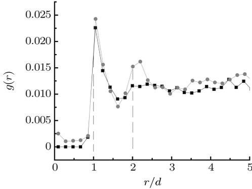
**Fig. 2.** Radial distribution function  $g(r)$ , where black squares are for cells of 2 to 8 layers of particles, gray circles for cell of 10 layers of particles; the vertical dashed lines correspond to the expected positions of the peaks in each of the phases.
