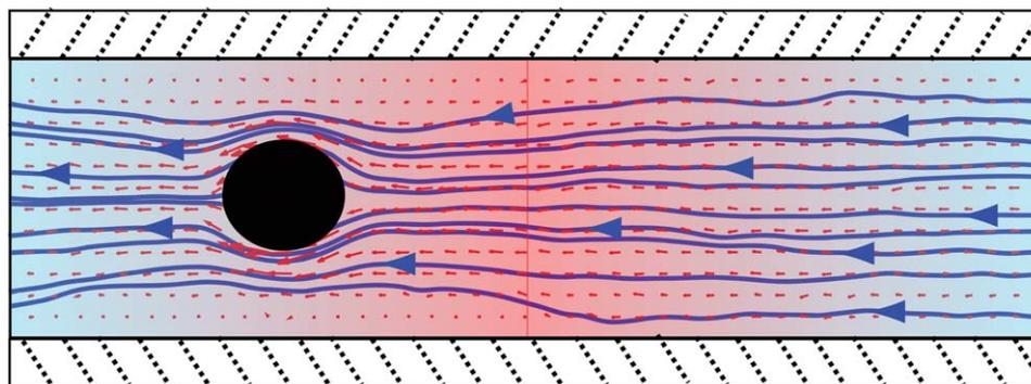
**Fig. 9** Single-particle thermophoretic pump. Thermophilic colloidal particle confined between parallel walls, with both extremes of the tube connected by PBCs, and larger temperatures in the tube center. Given that the colloid is thermophilic and has the hot layer on its right, the solvent continuously flows from right to left.
