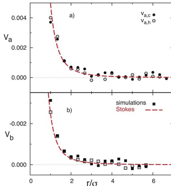
**Fig. 6** Velocity field around a drifting thermophoretic particle as a function of distance from the particle, with the positive direction toward the hot side. Symbols refer to the simulation results, lines to the theoretical calculation from eqn (4). (a) Velocity field  $V_a$ , solid and open symbols correspond to  $V_{a,c}$  and  $V_{a,h}$ , respectively. (b) Velocity field  $V_b$ .
