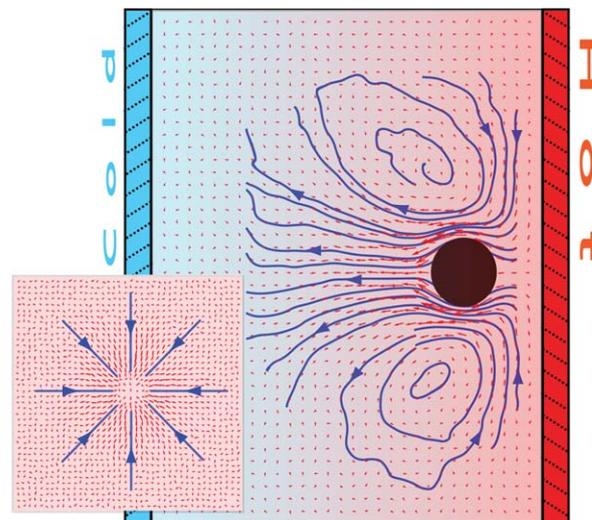
**Fig. 7** Cross-section of the flow field around a thermophilic particle fixed in a near-wall environment. The inset shows the velocity field in a plane parallel to the walls and between the colloid and the hot wall.
