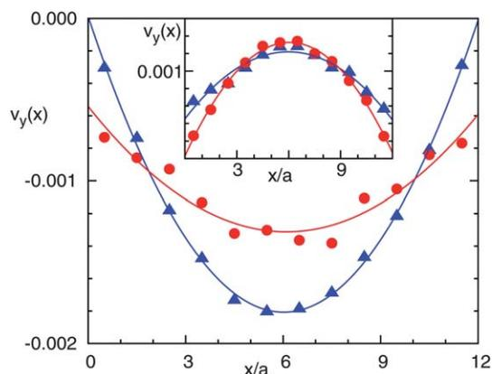
**Fig. 10** Velocity parallel to the walls and between them for the flow in Fig. 9. Triangles correspond to the average profile in a bin  $5a$  wide just on the right of the cold layer. Circles relate to a bin  $5a$  wide just on the left of the cold layer. Lines refer to a parabolic fit. The inset corresponds to the velocity profile in the same layers but for a thermophobic colloid.
