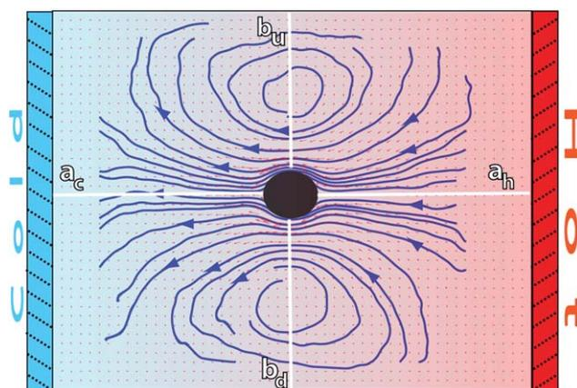
**Fig. 1** Cross-section of the flow field induced by a thermophilic colloid fixed between parallel cold and hot walls. Small red arrows indicate the flow velocity direction and intensity, while the thick blue lines correspond to the flow stream lines. The axes where the flow velocities are quantified in Fig. 2 are displayed here in white.
