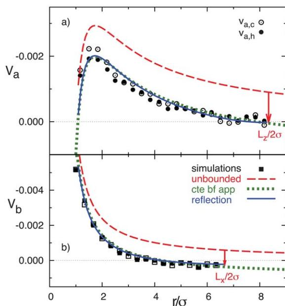
**Fig. 2** Flow velocity as a function of distance from the colloidal center. Symbols correspond to simulation results, dashed lines to the theoretical calculation in eqn (3), dotted lines to the constant backflow approximation, and solid lines to theoretical calculation with the reflection method. Arrows indicate the position of the system boundaries. (a) Velocity in axis *a*. (b) Velocity in axis *b*.
