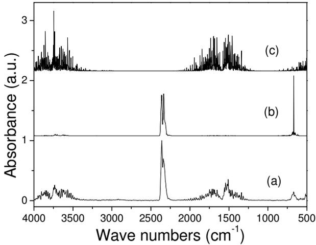
Fig. 5. FTIR spectra: (a) Gases vaporized at 120°C of 80°C dried LTO powder; (b) CO<sub>2</sub>; (c) water.
