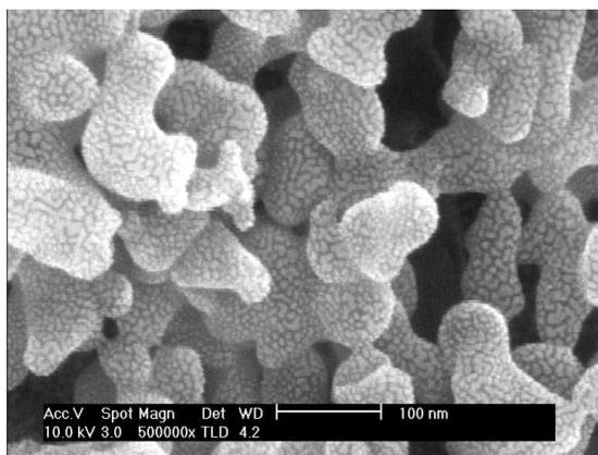
Fig. 1. SEM photographs of La-Ti-O (LTO) nanoparticles dried at 120°C. The light island shape spots on the surface of LTO particles are Aurum particles sprayed to enhance the conductivity of LTO particle for SEM measurement.
