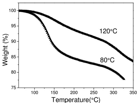
Fig. 4. TG curves of LTO particles dried at  $80^{\circ}\text{C}$  and  $120^{\circ}\text{C}$ .
