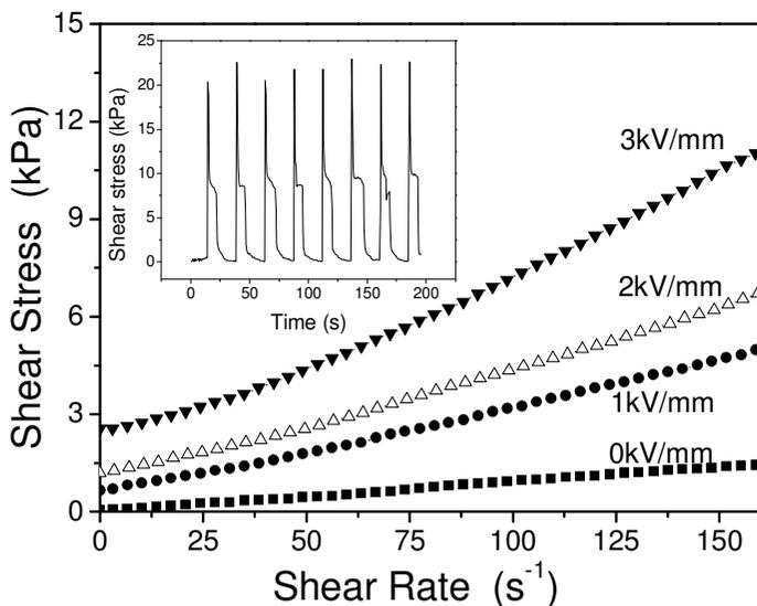
Fig. 3. The shear stress versus shear rate of the sample dried at  $120^{\circ}\text{C}$  with volume fraction of 45% at different electric field. Inset is the shear stress in an on/off mode of 3 kV/mm field at shear rate  $3.6\text{ s}^{-1}$ .
