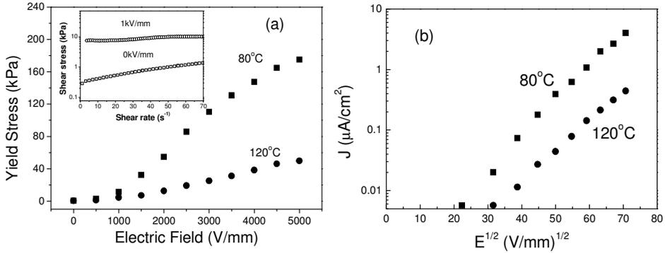
Fig. 2. (a) The relation of yield stress versus electric field (b) the behavior of current densities versus sqrt( $E$ ) of ER fluid for the La-Ti-O (LTO) powder dried at 80°C and 120°C with the volume fraction about 60%. The inset of Fig. 2(a) shows the shear stress versus shear rate at zero field and 1 kV/mm for the sample dried at 80°C.
