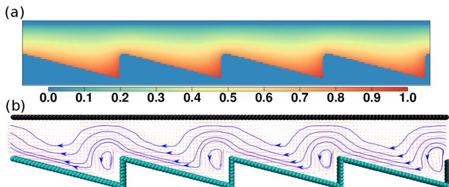
FIG. 7. (a) The steady-state relative concentration distribution of species B,  $\rho_B/\rho$ , and (b) the diffusio-osmosis induced flow field in the ratchet channel, with  $L_x = 31$ ,  $L_y = 20$ , and  $H = 8$ . Here, the transition  $A \rightarrow B$  uniformly occurs at the bottom wall with  $Pr = 0.55$ , and  $B \rightarrow A$  at the top wall with  $Pr = 0.1$ .
