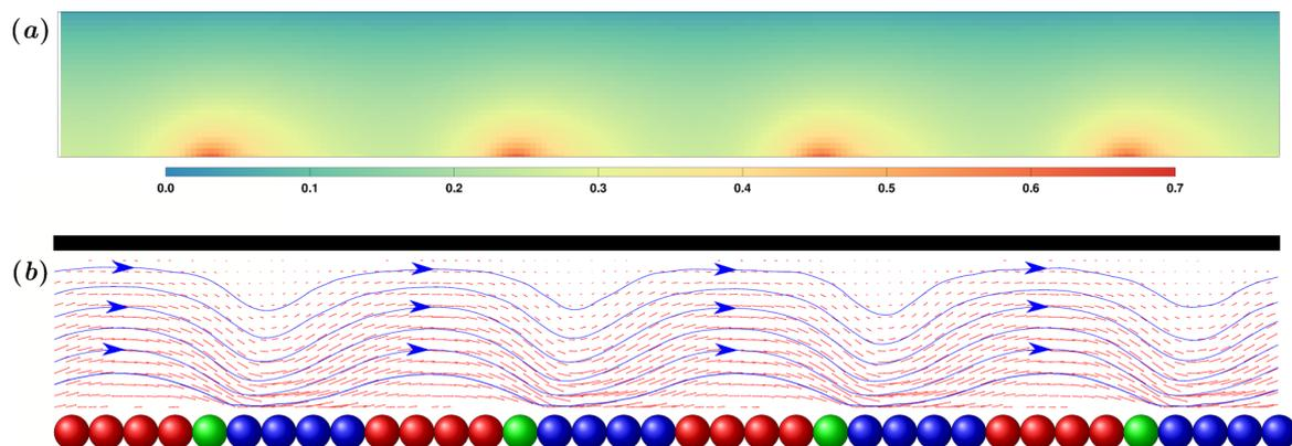
FIG. 3. Typical steady-state concentration distribution of species B (a) and flow field (b) in the planar channel of Fig. 1(a). B-particle concentration in (a) is measured in molar fraction,  $\rho_B/\rho$ ; and the blue lines in (b) refer to the streamline. Here,  $U_{3B} = a(12,1)$  and  $L_y = 16$  are used, and the transition probabilities of particles in the source and sink regions are set as  $Pr = 0.55$  and  $0.1$ , respectively.
