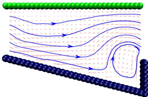
FIG. 8. Flow field induced by a chemical gradient in a ratchet channel, with the reaction  $B \rightarrow A$  at the bottom wall and  $A \rightarrow B$  at the top wall. Here, the bottom sawtooth wall acts as both B-sink and the driving part, and is drawn in dark blue. Other system parameters are the same as those of the ratchet channel in Fig. 7.
