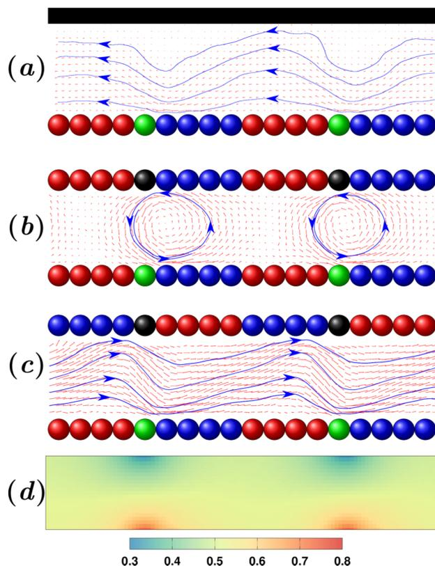
FIG. 4. Flow field in the planar channel of different boundaries. (a) The configuration is the same as that of Fig. 3 but uses  $U_{3B} = r(3,1)$  instead of  $a(12,1)$ . (b) The bottom and top walls are symmetric with respect to the central axis of the channel, as depicted in Fig. 1(b). Here,  $U_{3B} = a(12,1)$  is used. Systems (c) and (b) only differ in the position of 3 and 4-type beads of the top walls. (d) Steady-state concentration distribution of species B in the systems of (b).
