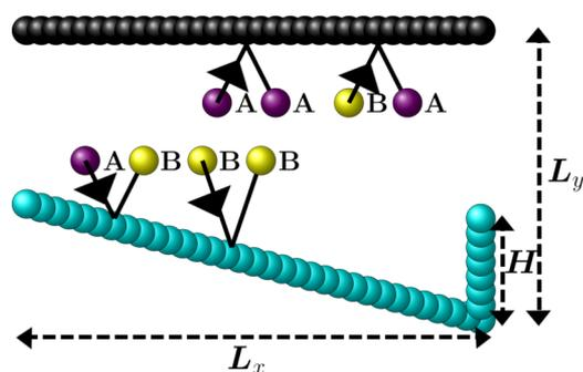
FIG. 2. Schematic diagram of ratchet channel. The whole sawtooth wall corresponds to the source of species B and the flat wall to the sink.  $L_y$ ,  $L_x$ , and  $H$  denote the dimensions of a driving unit, which are, respectively, the channel width, and the sawtooth length and height.
